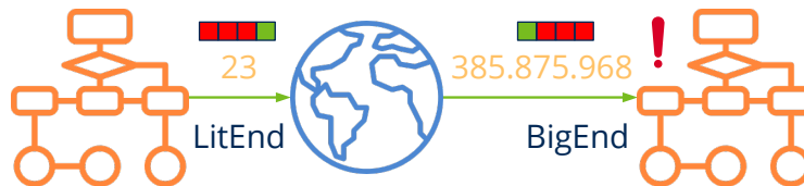
Figure 15.22: We must take into account endianness when sharing data between machines of different architecture.
