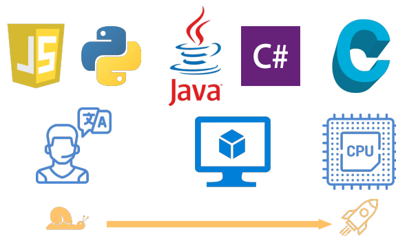
Figure 2.4: Interpreter, virtual machine, and binary code. The closer we get to machine language, the more performance we will get from the software.
