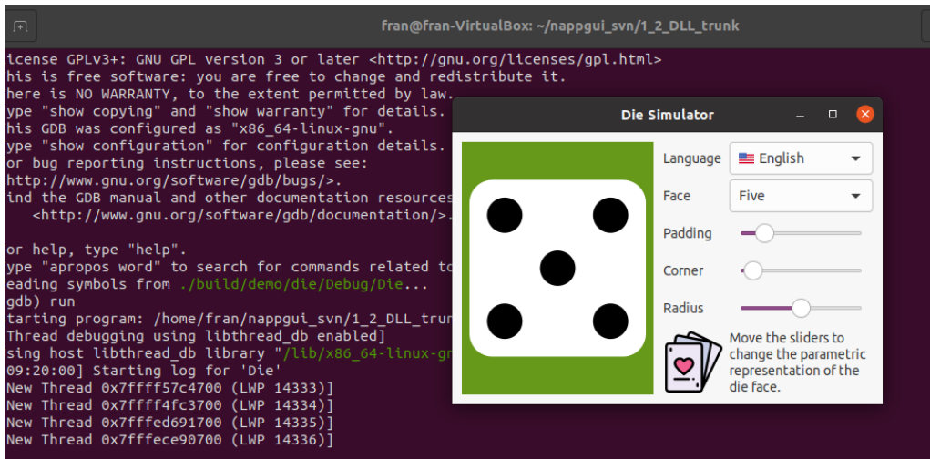
Figure 8.15: Debugging Die with GDB from the terminal.
